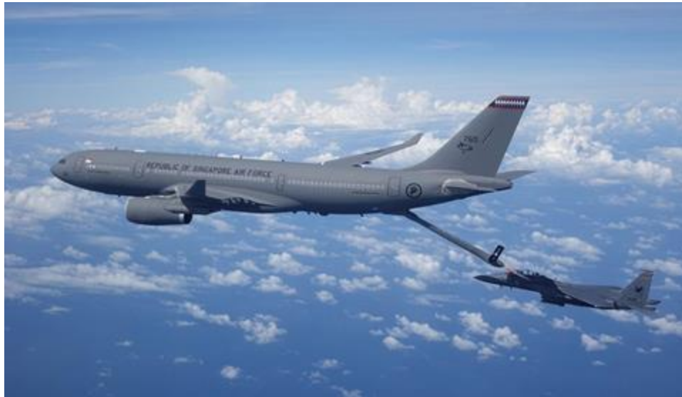
Figure A-3. RSAF A330 MRTT in an Aerial Refueling Operation with an RSAF F-15SG
